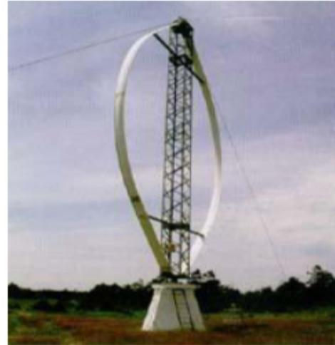
Figure I.3: Eolienne de Darrieus.
