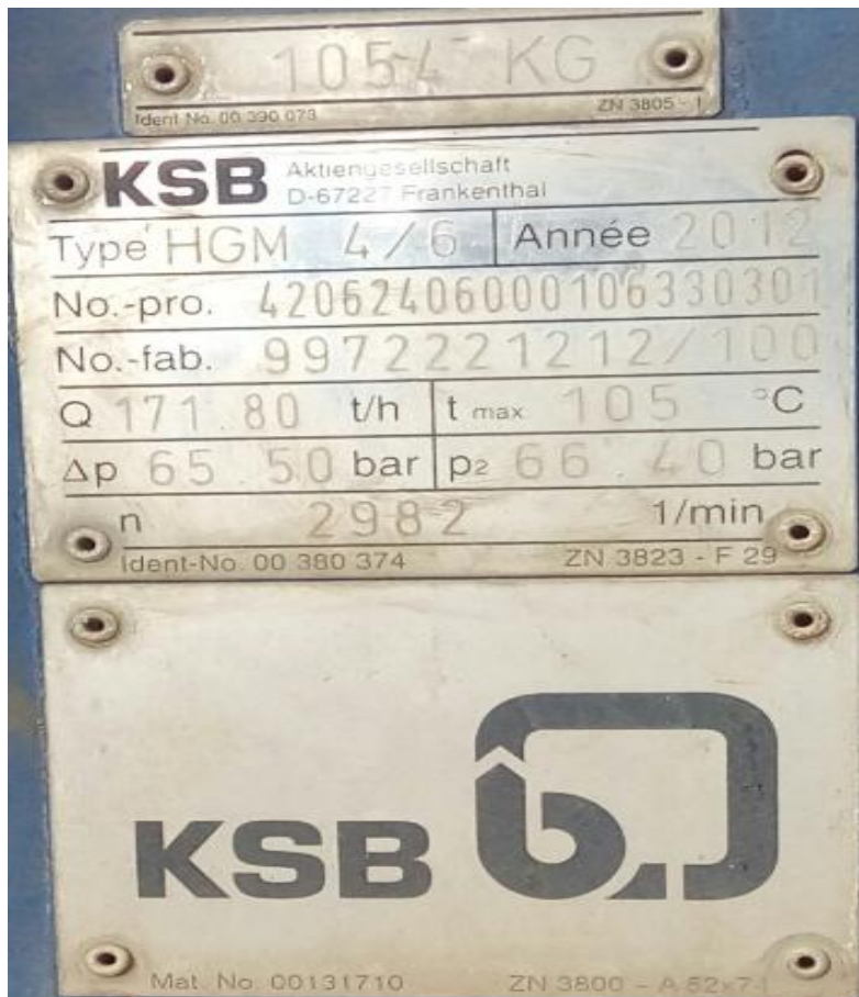
Figure (annexe. c): pompe multicellulaire KSB HGM 4/6.
