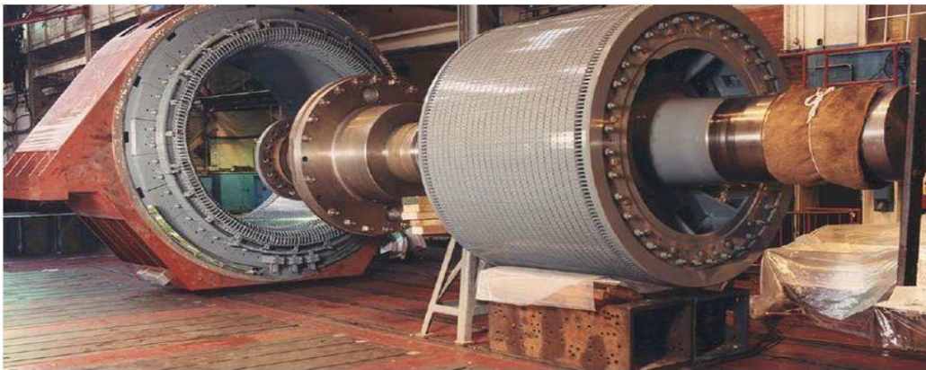
Figure I.1 : Machine asynchrone de 4.7 MW, 45tr/mn [11]
