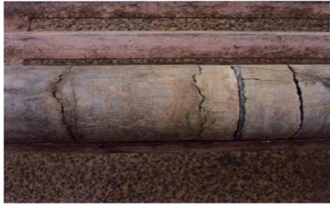
Figure II.13: Joints stylolithiques [puits OMLZ 36].
