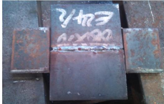
FIGURE 3.4 – Bridage des plaques.
