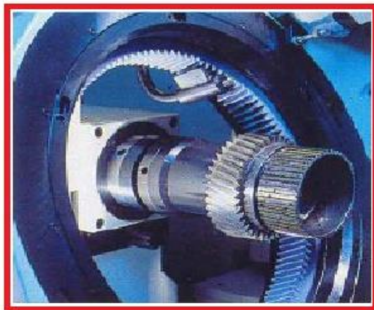
Figure II.10 : Rodage des dentures
