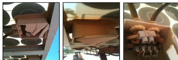
Figure 4. Effect of temperature and sand wind on junction box (station of MELOUKA).
