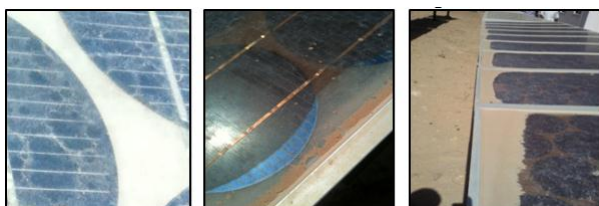
Figure 1. Degradation of the optical properties of glass (station of MELOUKA).
