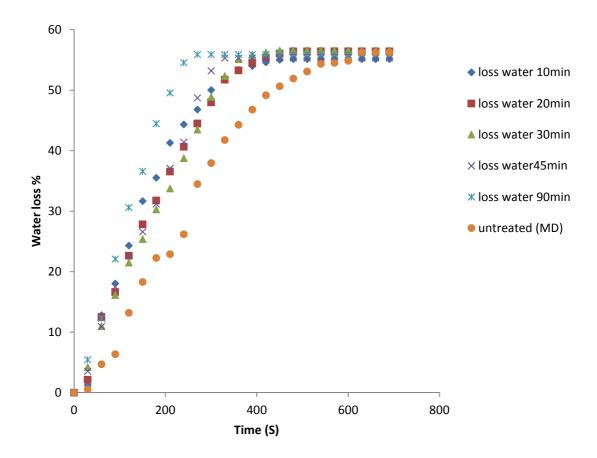
**Figure n°8:** Influence of ultrasonic time on the dehydration kinetics process at 700 W of Myrtle pericarp.
