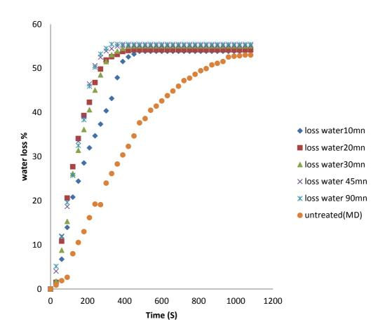
**Figure n° 7**: Influence of ultrasonic time on the dehydration kinetics process at 500 W of Myrtle pericarp.
