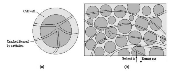
Figure n° 3: The mechanism of cell wall disruption (a) breaking of cell wall due to cavitation
