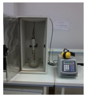
Figure n° 6: Ultrasound assisted extraction system.
