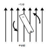
Figure n° 2: Movement of a dipole in an electric field (Singh and Heldman, 2001).
