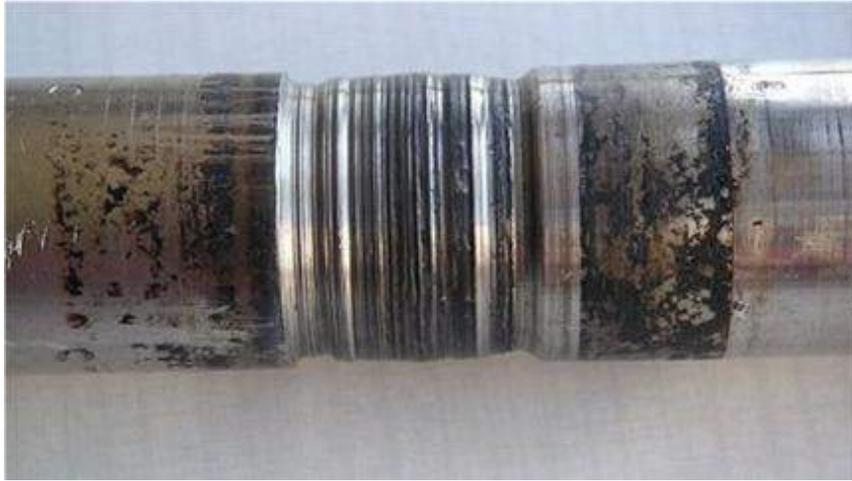
**Figure I.14 :** *usure abrasive* [29].
