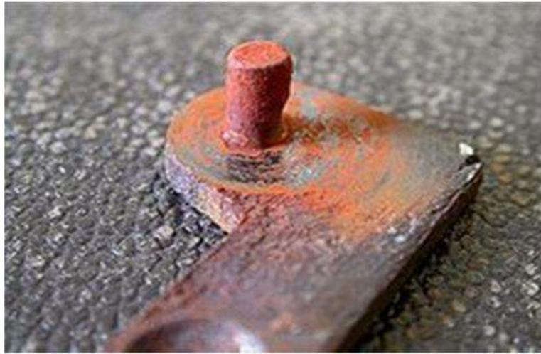
**Figure I.16 :** *usure de corrosion* [29].
