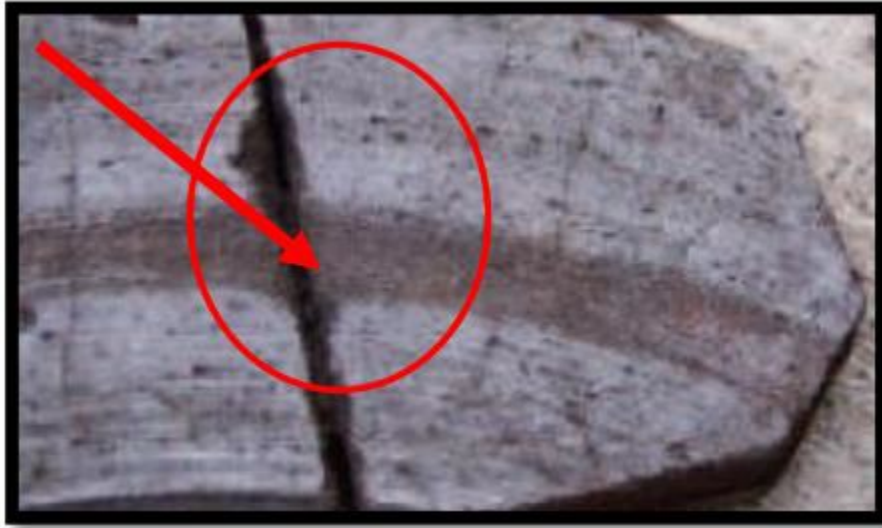
Figure.I.36: Plaquette a usure non- uniforme.
