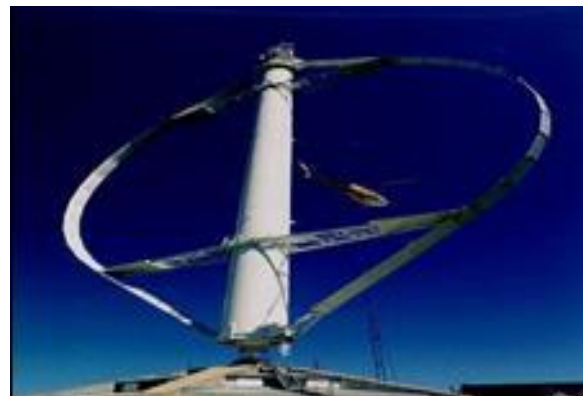
Figure II.15: Éolienne de type Darrieus [14]
