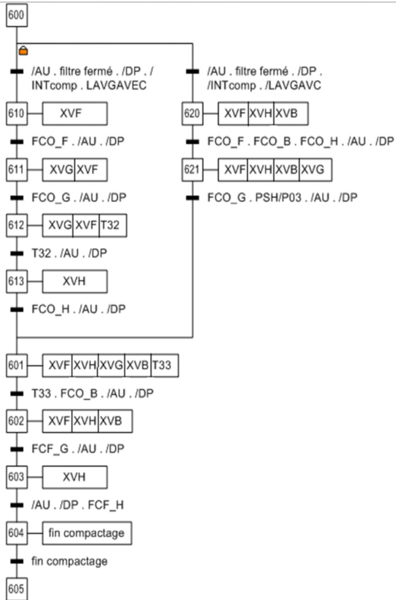
Figure III. 7 GRAFCET de compactage
