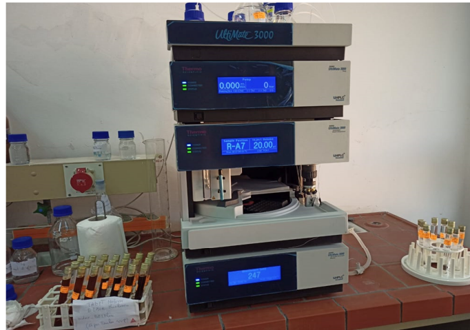
Figure 17 : appareil durnex ultimate 3000 (HPLC)
