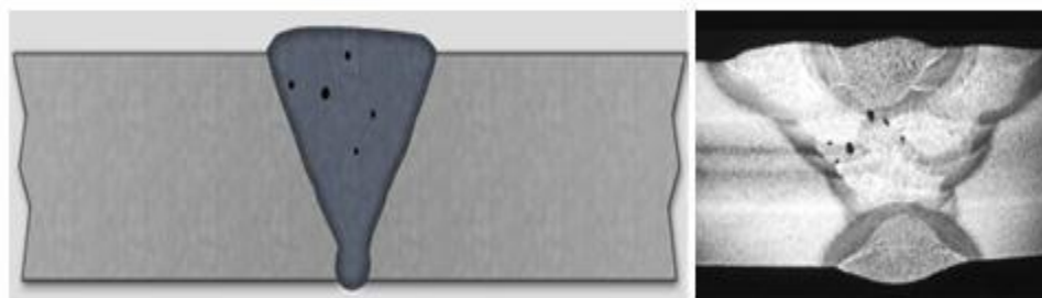
Figure I.24: inclusions gazeuses porosités uniformes.
