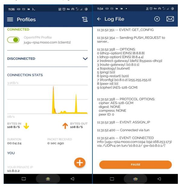
Figure IV.37: screenshot of smartphone connected to the master RPI's VPN server
