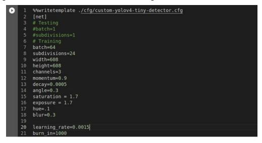
Figure IV.6: Python code shows writing YOLO configurations used to train the mask model
