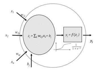
Figure II.10: A presentation of neuron : "wij" weights, "bj" biases, "xn" inputs, and "yi" output
