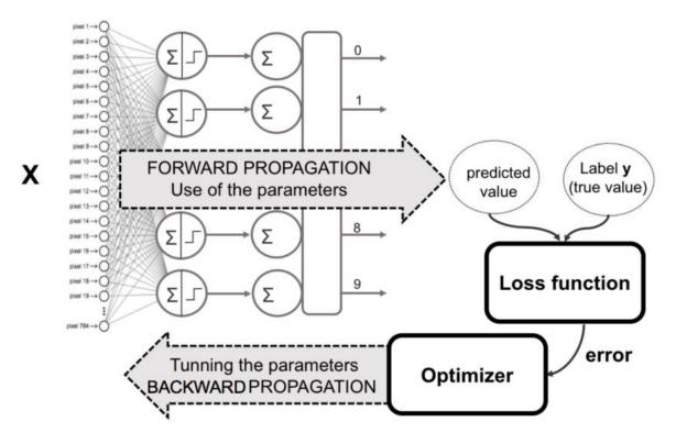
Figure II.11: Back-propagation and forward-propagation process
