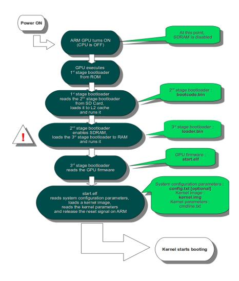
Figure F.1: The boot sequence of the Raspberry Pi in general
