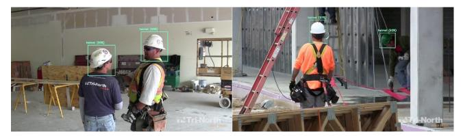
Figure IV.20: Examples of detected frames on Raspberry-Pi Client while using hard-hat detection
