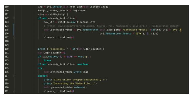
Figure IV.27: Python code shows generating a video files from received frames.
