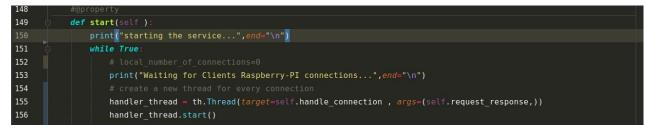
Figure IV.24: Python code shows using multithreading for each client connection
