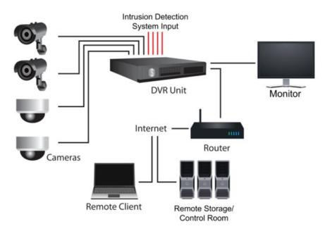
Figure I.1: Typical surveillance system components
