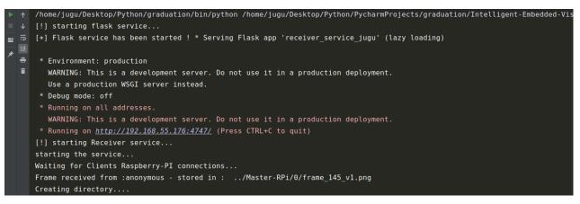
Figure IV.31: Python output logs shows the execution of the services.
