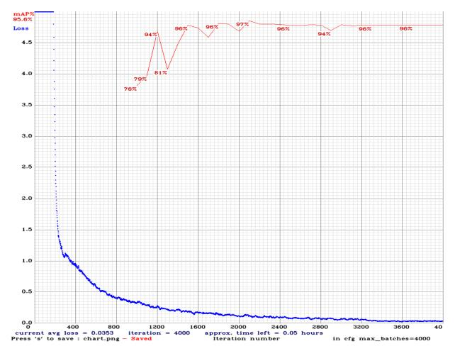
Figure IV.4: Learning curve for the Thermal-Infrared person-dog model using darknet framwork
