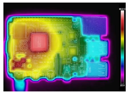
Figure III.5: Picture from thermal imaging camera and Raspberry Pi 4B
