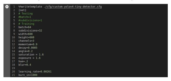
Figure IV.9: Python code shows writing YOLO configurations used to train the hard-hat model,
