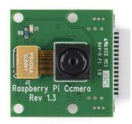
Figure III.8: A picture of Raspberry Pi Camera Module Rev 1.3 - 5 Megapixel
