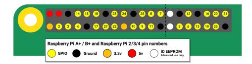
Figure III.4: GPIO Connector Pinout
