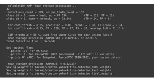
Figure IV.8: Performances of the mask detection model on darknet
