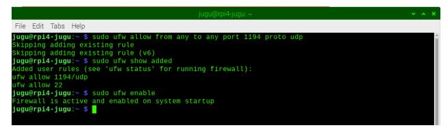
Figure IV.36: Raspberry pi firewall configuration
