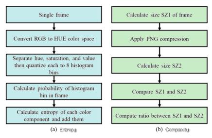
Figure IV.12: Computing entropy (a) and complexity (b) score from a single input frame
