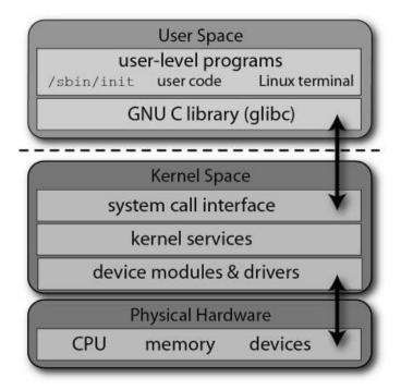
Figure III.9: The Linux user and kernel space architectures
