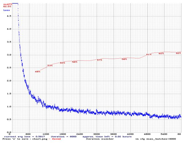
Figure IV.10: Learning curve for the hard-hat detection model using darknet framwork
