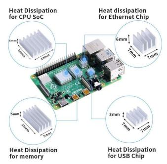
Figure III.6: Raspberry-Pi with heatsinks attached to it.
