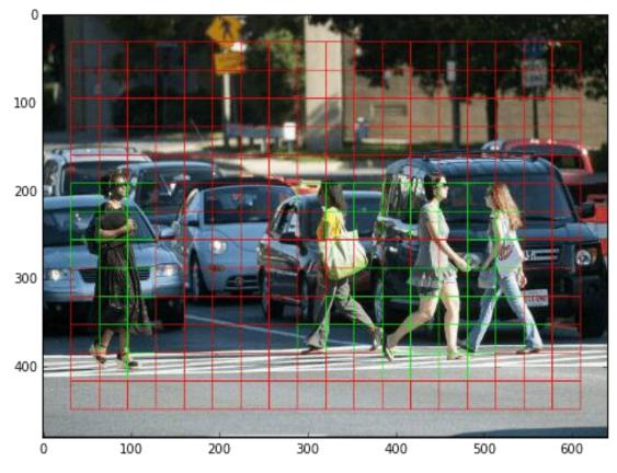
Figure II.14: How an input image is divided into grids in YOLO
