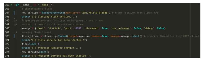
Figure IV.30: Python code shows running Flask on separate thread on port 4747.
