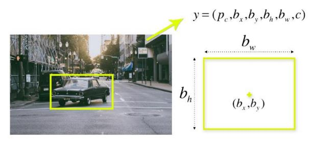
Figure II.15: An image shows an example of a bounding box in yollow color
