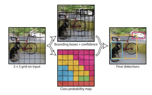
Figure II.17: Combination oh the 3 techniques to produce the final detection in YOLO
