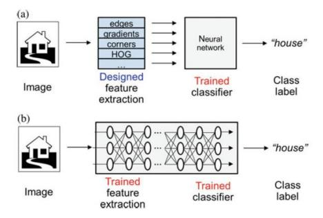
*Figure II.13*: Comparing the (a) classical approach to machine learning using handcrafted fetaures to the (b) deep learning operating on raw inputs.
