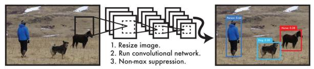
Figure II.13: YOLO Detection System [8]
