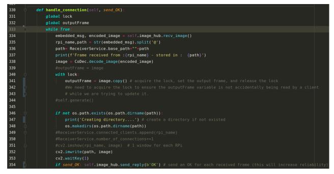
Figure IV.25: Python code shows handle\_connection function
