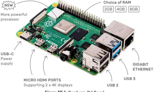
Figure III.3: Raspberry-Pi4 Board
