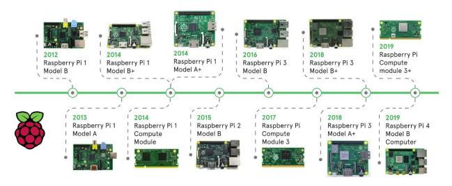
Figure III.2: The evolution of Raspberry-Pi models
