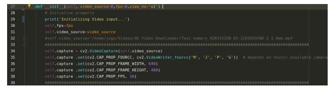
Figure IV.18: Python code shows configuration of OpenCV instance
