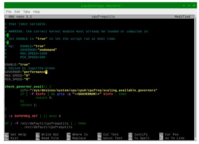
Figure III.12: Editing the cpufrequtils file to change the governor permanently.
