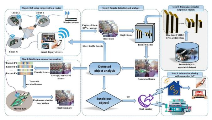
Figure IV.1: Overall system with different training steps, data acquisition, objects analysis and summary generation
