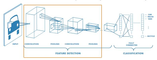
Figure II.9 : Basic CNN structure [6]
