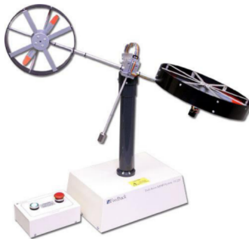
Fig. 1. Twin Rotor MIMO System.
