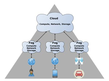
Figure 2.2: A Typical Fog Architecture [9]
