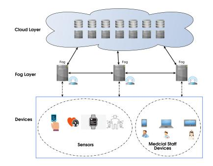
Figure 5.1: A Typical e-health Architecture [9]
