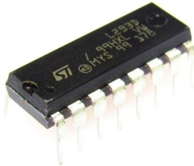
Figure II.5: Circuit intégré L293D
