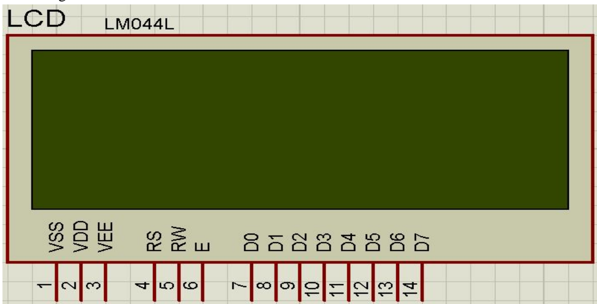
Figure III.17: L'afficheur LCD LM044L 20x4.
