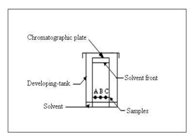
Figure 5 : A typical TLC system
