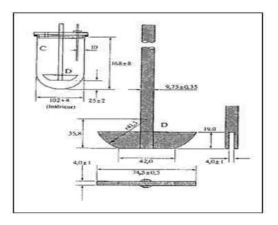
Figure 10 : Paddle Apparatus
