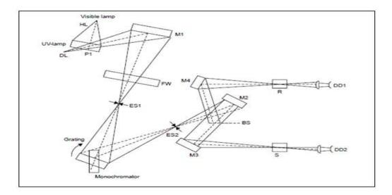
Figure 8 : Schematic representation of the optical system in a double-beam spectrophotometer Model lambda-2 micrometer controlled UV-Visible spectrophotometer (Perkin-Elmer) The various components of Figure 8 are stated below:
