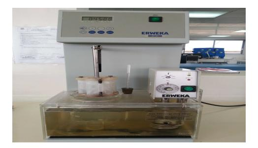
Figure E: Deletion apparatus, ERWEKA ZT31
