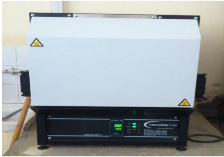
Figure 8 : photo de Four de calcination.
