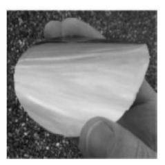
Figure 2.4: Photograph of a 14  $\mu m$  thick epitaxial silicon film on top of a 1.5  $\mu m$  thick QMS film, transferred to a plastic foil.
