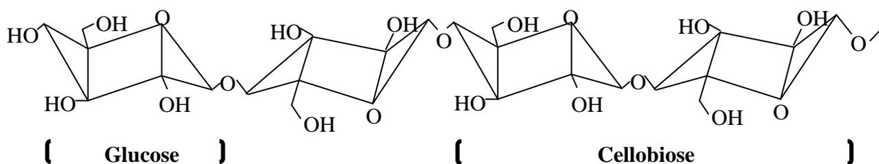
Fig.1: Molecular chain structure of cellulose [8]
