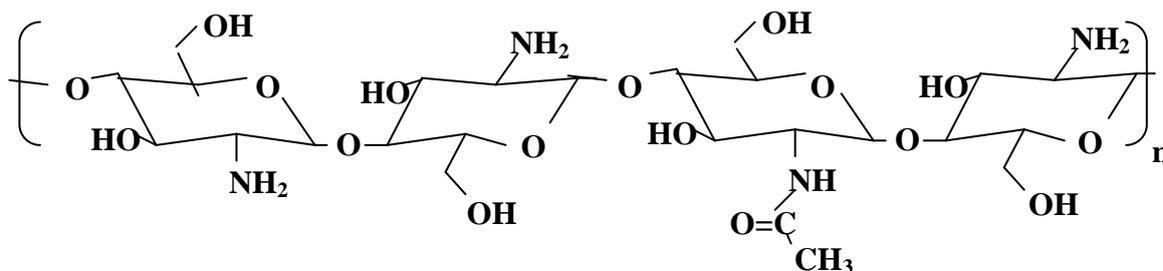
Fig. 4: Chitosan chemical structure [19]
