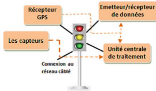
FIGURE 1.6 – WAVE RoadSide Unit. [12]
