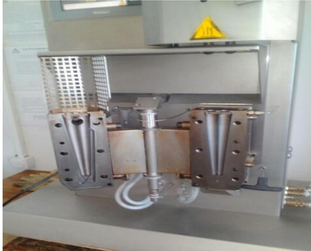
**Figure II.3 :** Mini-extrudeuse bis-vis de type micro compounder DSM Xplore modele 2005.
