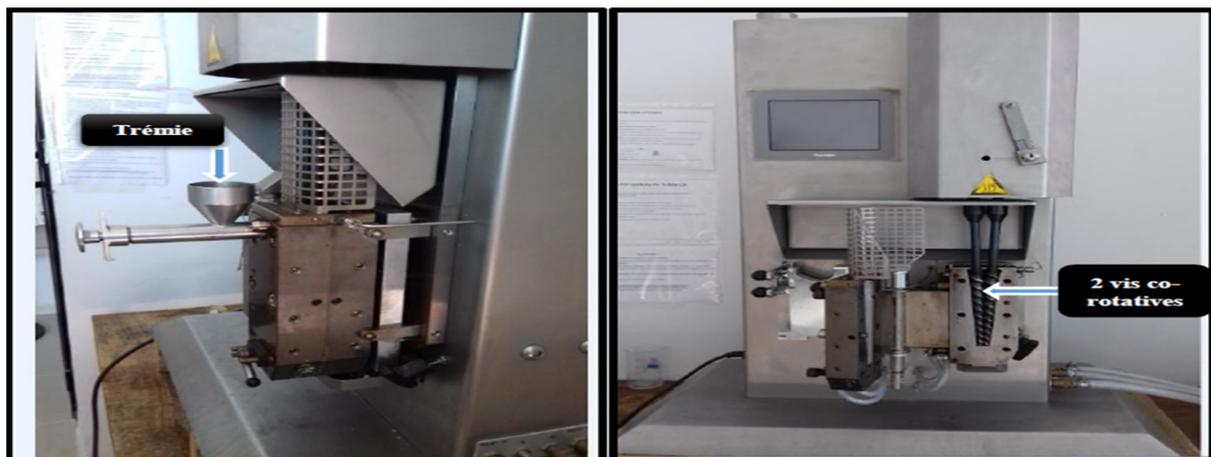
**Figure III. 6.** Mini-extrudeuse bi-vis micro compounder DSM Xplore.
