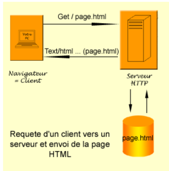
Figure I. 2 - Architecture d'une application 2 tiers [5].
