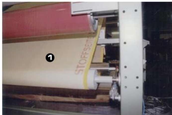
Figure II.5: Bande de transport du tissu.
