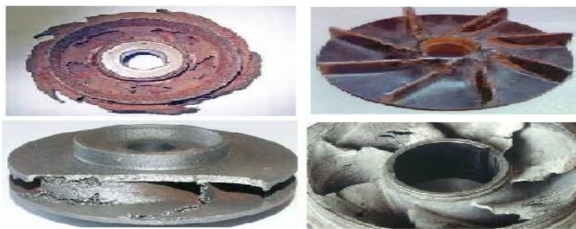
Figure I.8: Cavitation des pompes.
