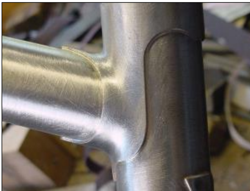
Figure II.12 Soudage des tubes
