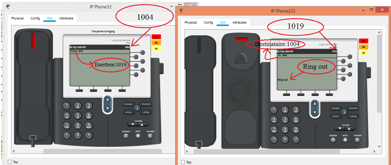
Figure 4.22-Test entre IP Phone225et IP phone 32.
