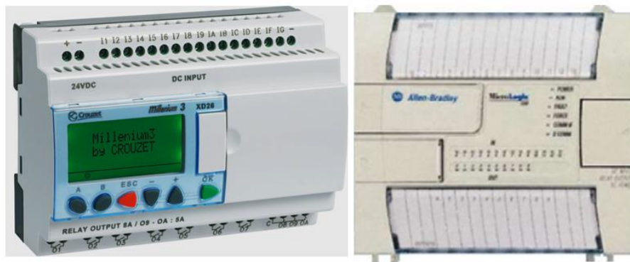
Figure I.2 : Automate compact (Crouzet, Allen-bradley).
