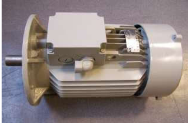
Figure II.1 : machine asynchrone de 8KW [18]
