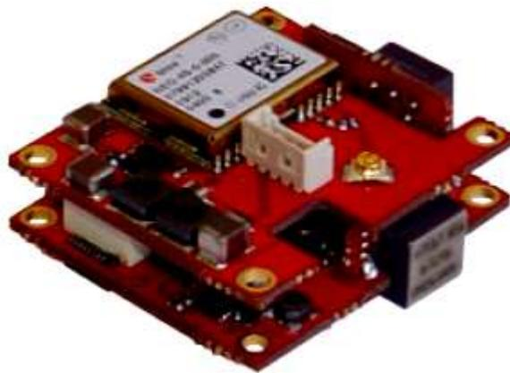
Figure I.26. Centrale inertielle IMU [33].
