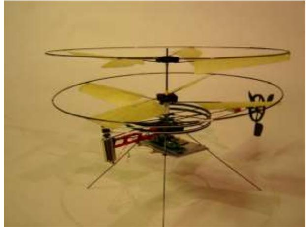
**Figure I.4.** Micro drone: Proxflyer [13].
