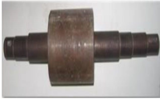
Figure I. 5 -Rotor massif lisse
