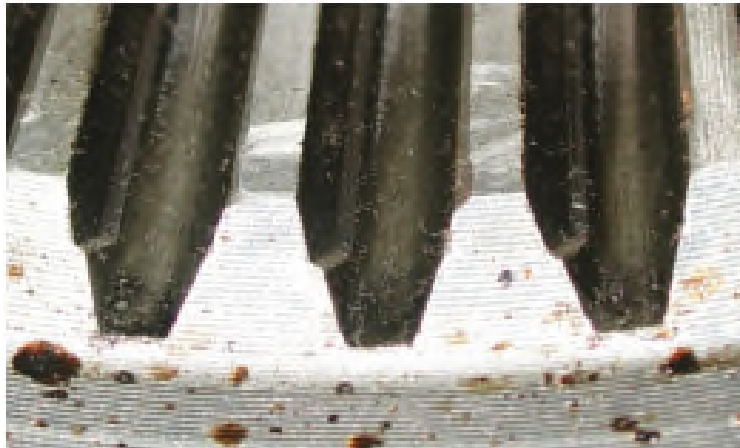
Figure I. 2 Usure abrasive "Engrenages"[02]
