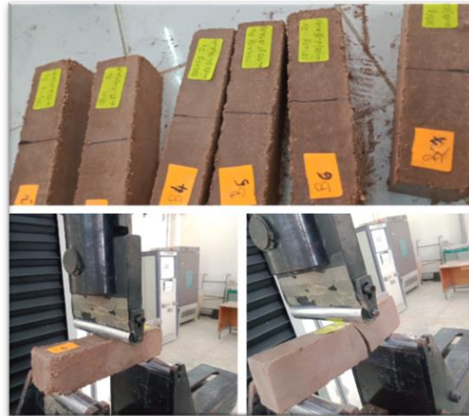
Figure 2. 27 : essai de traction
