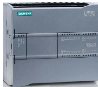
Figure III.4 : Automate programmable industriel S7-1200.
