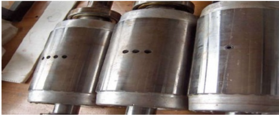
FIGURE 1.10 – Ruptures de barres
