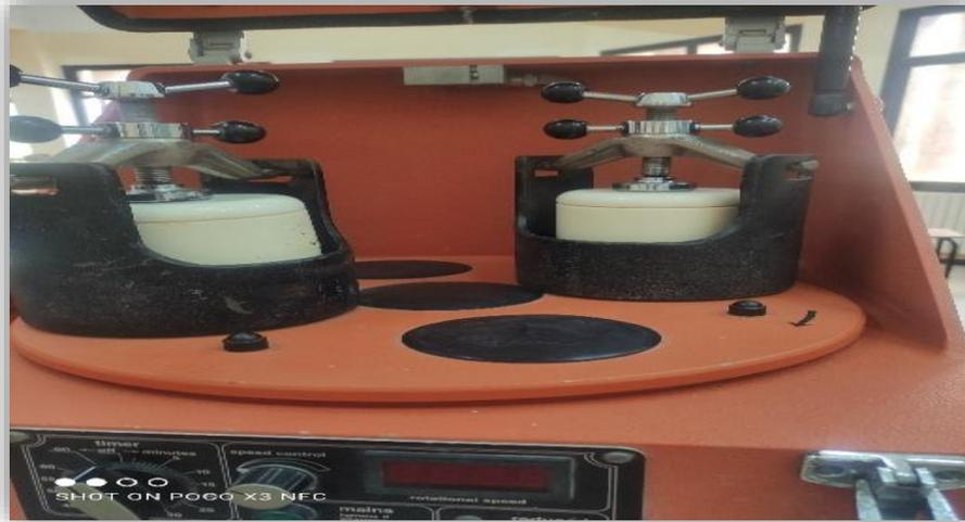
Figure III.6: Broyeur type RETSCH.
