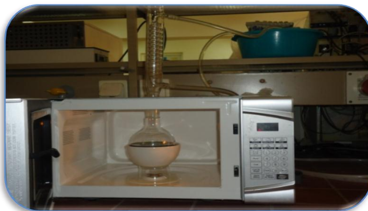
Figure 7: Microwave oven used for microwave-assisted extraction
