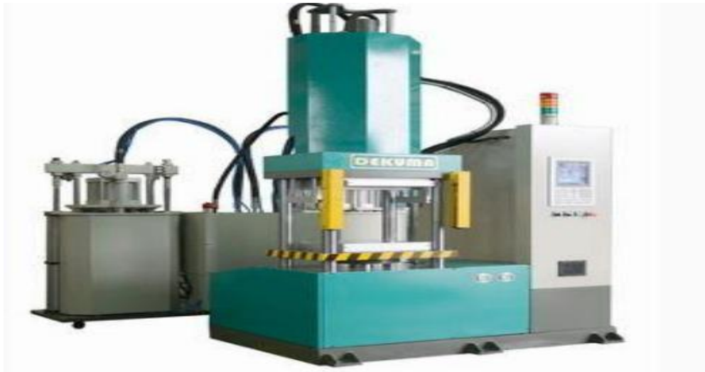
Figure I- 15: Presse à injection verticale.
