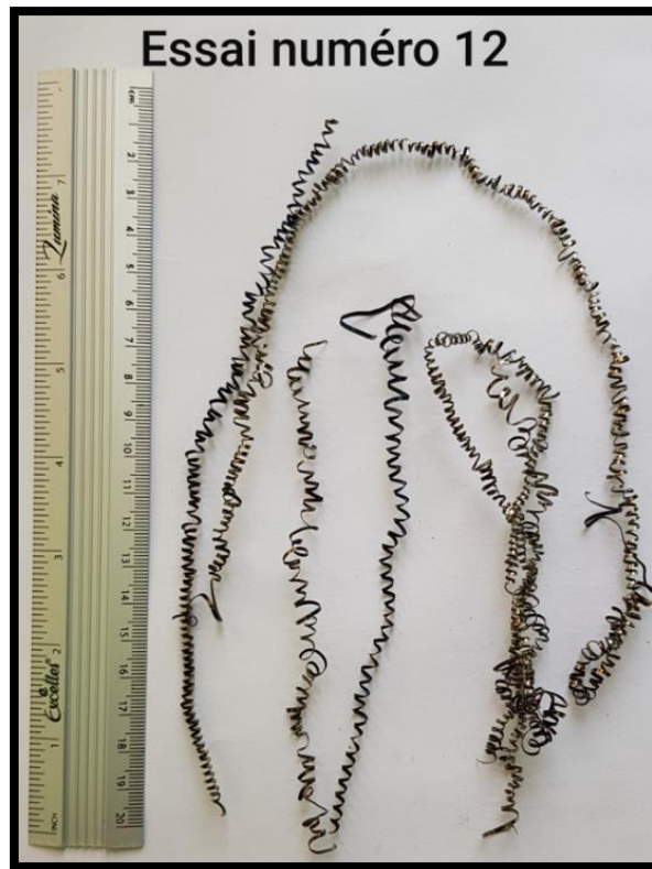
Figure IV. 38 : Copeaux tubulaires longs.
