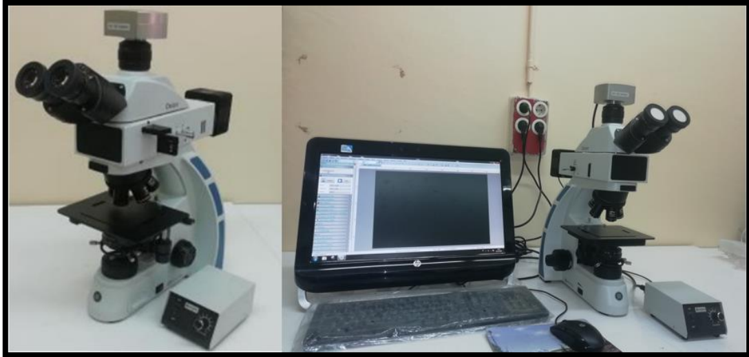
Figure III. 7 : Microscope optique OXION.
