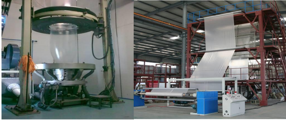
Figure III.2. Extrusion et coextrusion gonflage de films PEBD.
