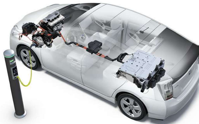
Figure I. 13 : Architecture Toyota Prius rechargeable
