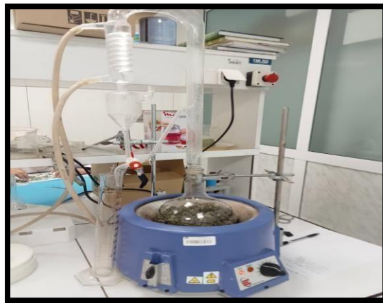
Figure 2 : Appareil hydro distillation de type Clevenger (CRD Saidal biotic)
