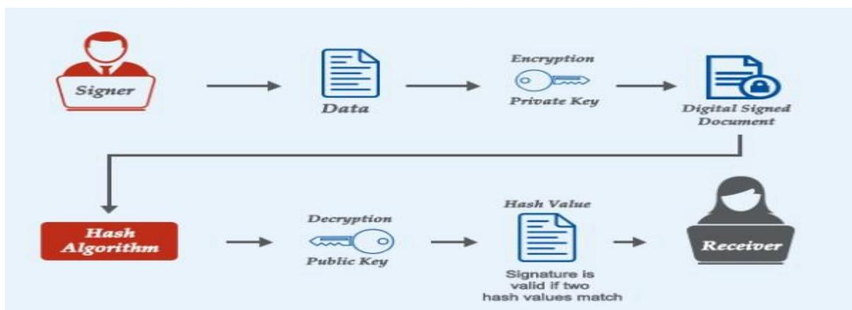
Figure 4 Process of signing smart contract [19]
