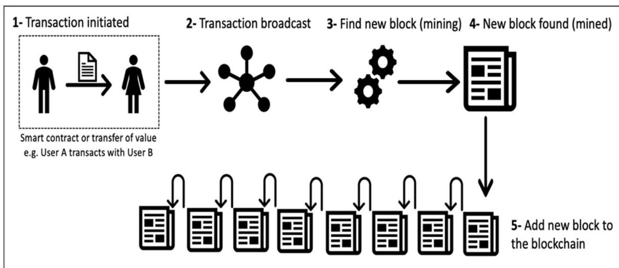
**Figure 3 steps involved in adding a new block to the blockchain**
