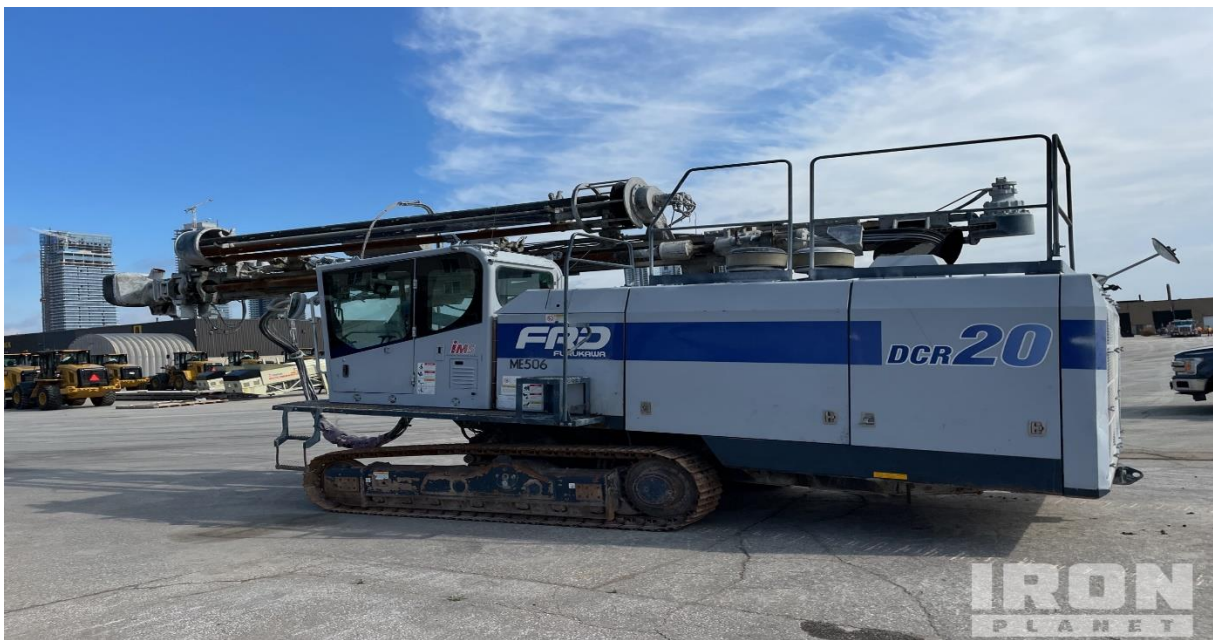
Figure II.6. La sondeuse Furukawa FRD DCR-20. [2]
