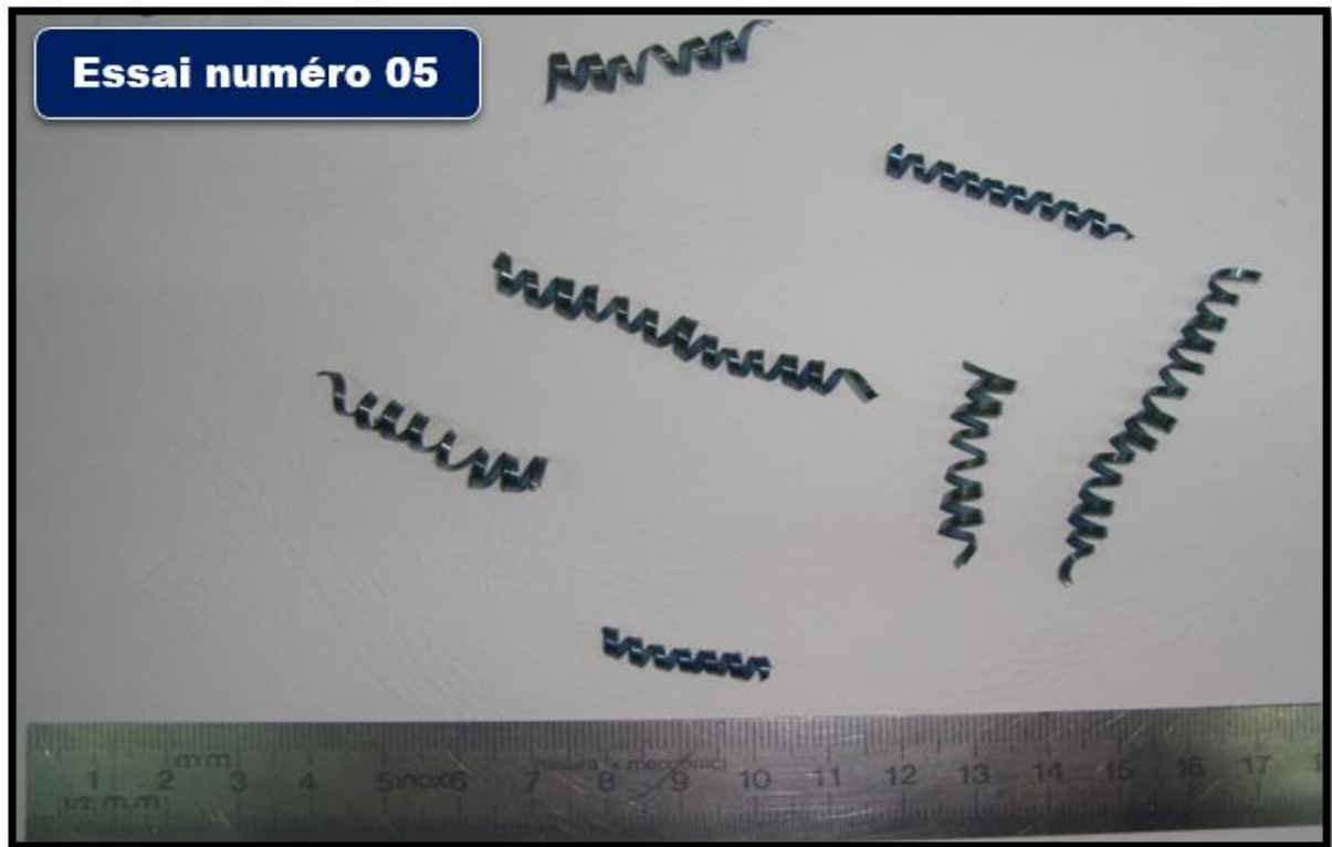
Figure 4.25 : Copeaux tubulaires longs.
