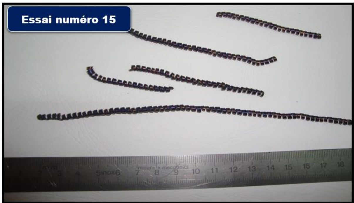
Figure 4.45 : Copeaux tubulaires longs.
