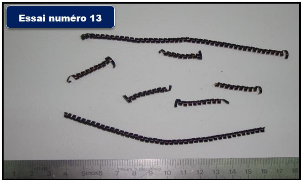
Figure 4.41 : Copeaux tubulaires longs.
