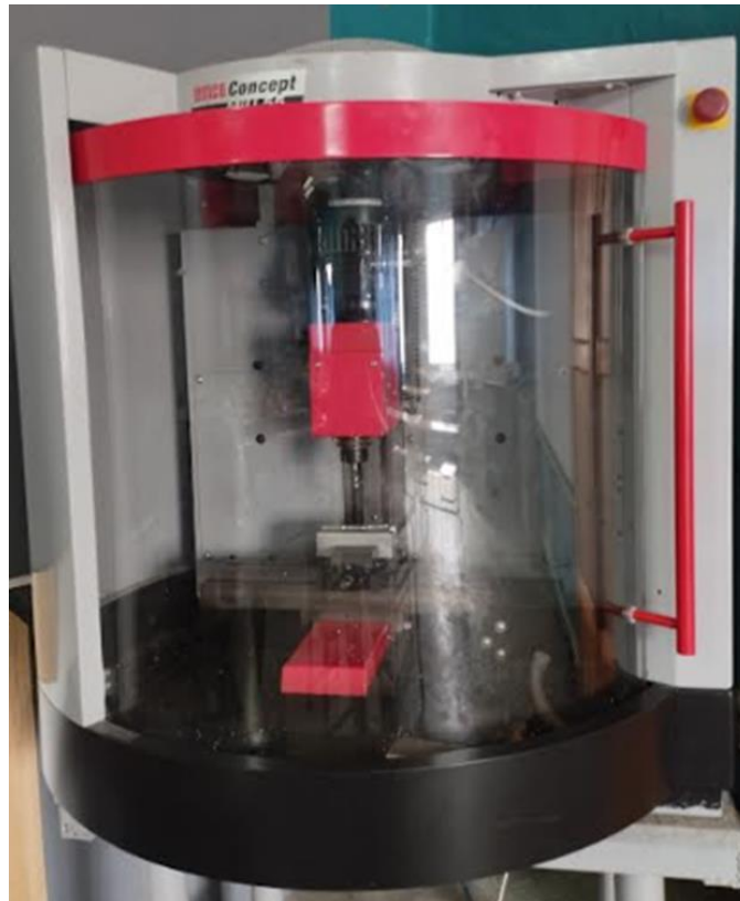
Figure III.7: Machine-outil emco concept mill 55 [15]
